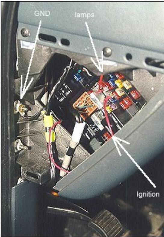
The photo on the left shows both the power and ground connections. The ground connection used is a stud that can be double-nutted with a 6mm nut with a crimon electrical connection. Both the gauge lamp grounds and the gauge ground connections are made at this point.
